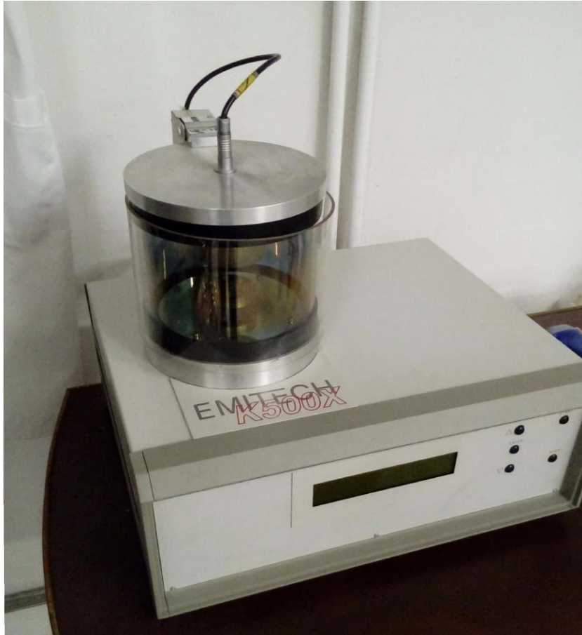
DC magnetron sputtering Au K500X (Quorum Technologies)
